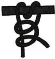
Round turn-and-two half hitches
